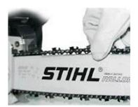
3. If the lower side of the chain does not hang away from the bar, but the chain can still be pulled away slightly, the tension is correct. You should also be able to lift the top side of the chain slightly (see picture). To prevent injuries from the sharp edges of the chain, you should wear protective gloves when doing this.
