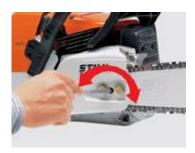
1. With the engine turned off, first loosen the securing screws of the chain cover with a combination wrench. To tension the chain, it is sufficient to only loosen these screws. Then turn the tensioning screw with the screwdriver end of the combination wrench (see picture).
